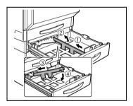
4 Slide the lateral guides to fit the size of paper to be loaded.
